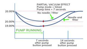
This graph depicts the change in reading with the pump time set to 7 seconds. With no needle and no filter, the reading drops to about 20%. With a needle and filter, the reading drops to about 19%. If you have a clogged needle and/or filter, the reading will drop to 10-16% and climb back up very slowly! If this happens, replace the needle and filter.
